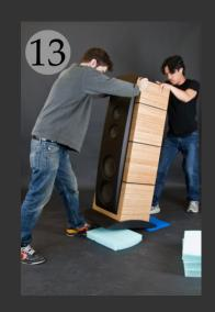
TIP SPEAKER FORWARD, REMOVE LARGE PIECE OF FOAM, REPLACE WITH RUBBER AND LOWER GENTLY.
