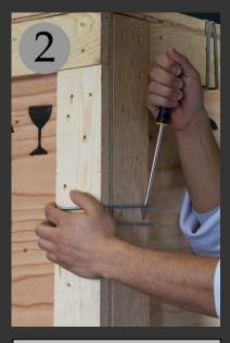
REMOVE THE METAL CLIPS FROM THE CRATE USING A FLAT HEAD SCREWDRIVER.
